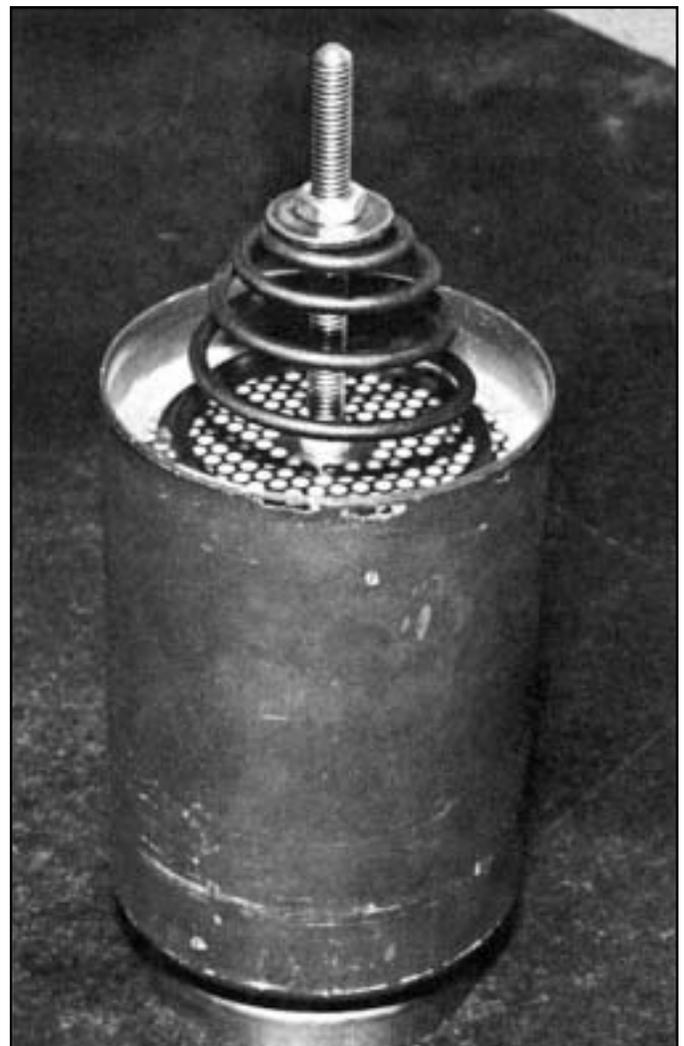
FIGURE 7 - REPLACEMENT DESICCANT CARTRIDGE
