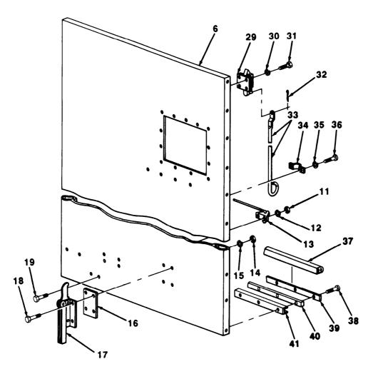
6. install holder assembly (13) on door (6) with two screws (19), new lockwashers (12), and nuts (11).
