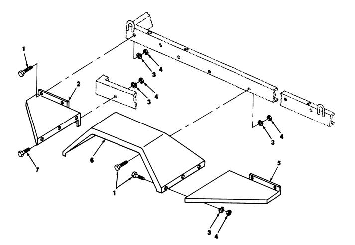
FIGURE 29. WATER TANK FENDERS AND EXTENSIONS (M107A1, M107A2, M107A2C).
