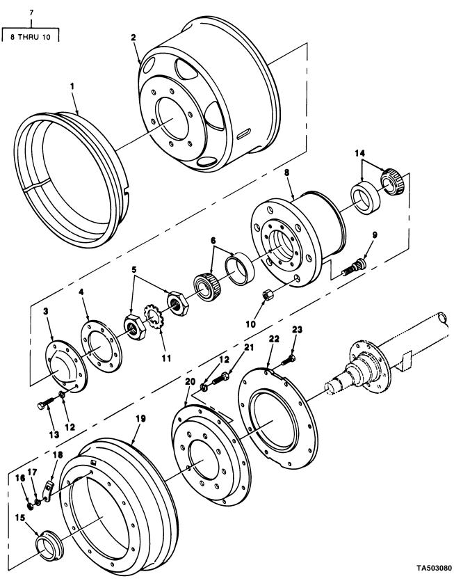
FIGURE 22. HUB AND DRUM ASSEMBLY (M103A1, M105A1, M107A1).
