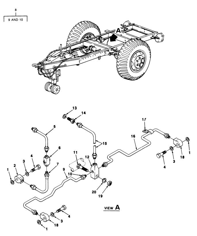
FIGURE 13, HYDRAULIC LINES, HOSES, AND FITTINGS (M103A1, M103A3, M105A1, M105A2, M107A1, M107A2, M107A2C, M448),
