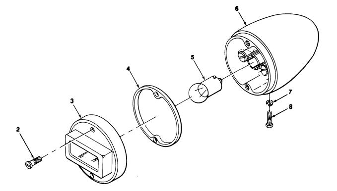
FIGURE 2. BLACKOUT STOPLIGHT (M103A3, M105A2, M105A2C, M107A2, M107A2C, M448),
