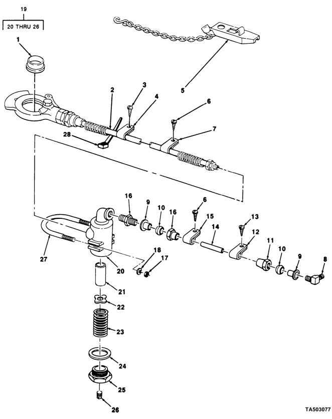
FIGURE 19. AIR LINES, HOSES AND FITTINGS (M103A1, M103A3, M105A1, M105A2, M107A1, M107A2, M107A2C, M448).
