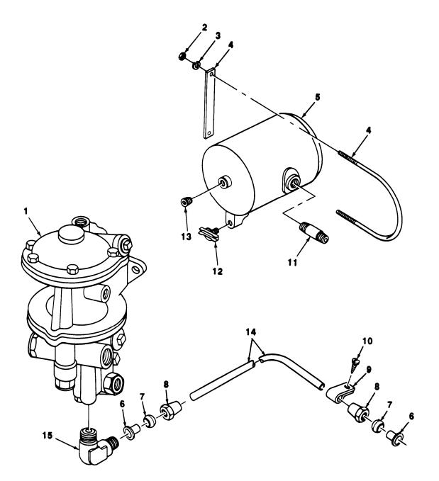
FIGURE 20. EMERGENCY RELAY VALVE AND RESERVOIR (M103A3, M105A2, M107A2, M107A2C, M448).
