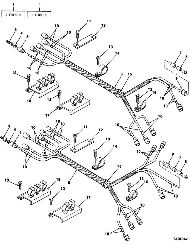
FIGURE 4. CHASSIS WIRING HARNESS.
