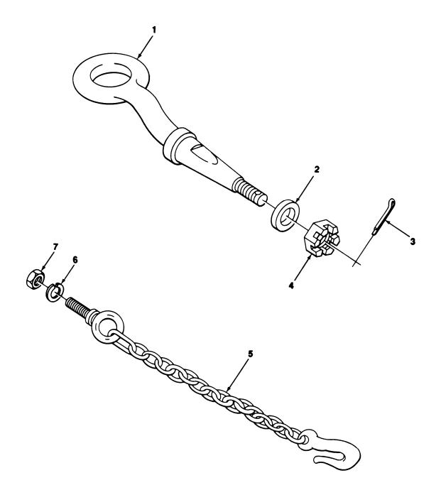
FIGURE 24. DRAWBAR RING AND SAFETY CHAIN.
