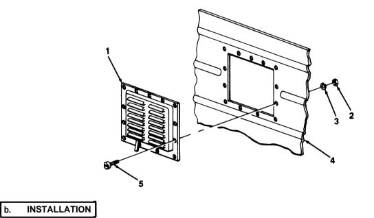
Position front ventilator (1) on front wall (4) and install 13 screws (5), new lockwashers (3), and nuts (2).
