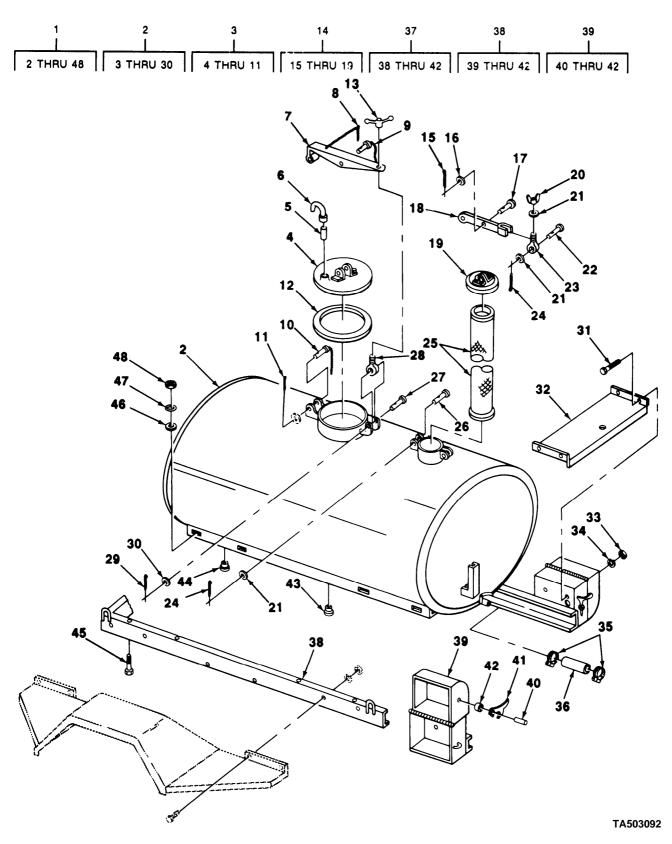
FIGURE 34. WATER TANK, TANK FRAME, AND RELATED PARTS M107A2, M107A2C).
