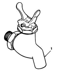
FIGURE 33. FAUCET ASSEMBLY (M107A1, M107A2, M107A2C).
