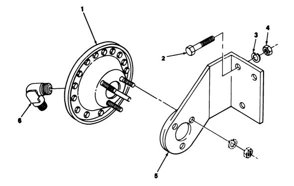
FIGURE 18. AIR CHAMBER ASSEMBLY (M103A1, M103A3, M105A1, M105A2, M107A1, M107A2, M107A2C, M448).
