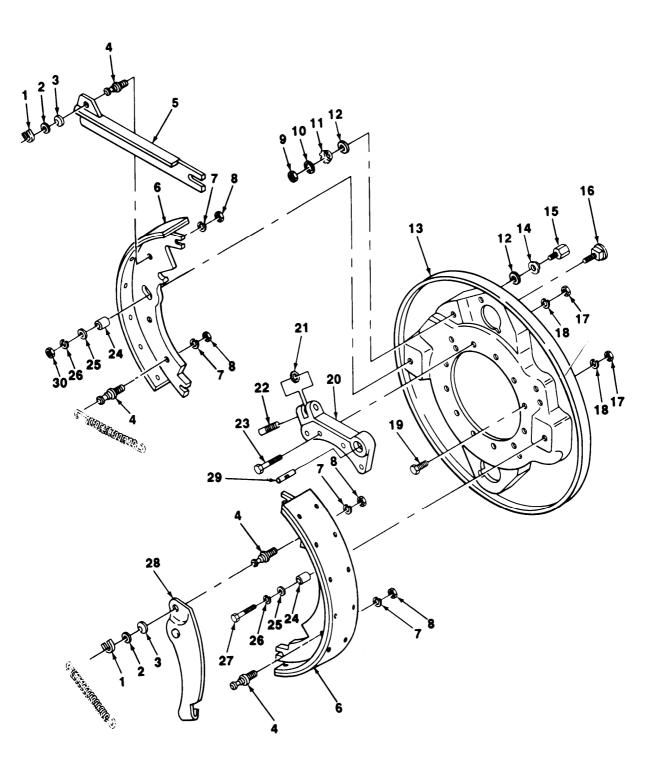
FIGURE 9. SERVICE BRAKES (M105A2C, M448, M103A3, M105A2, M107A2, M107A2C).
