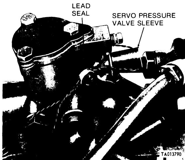
Figure 3-177. Installation of seal wire on fuel density compensator servo-pressure valve sleeve.
