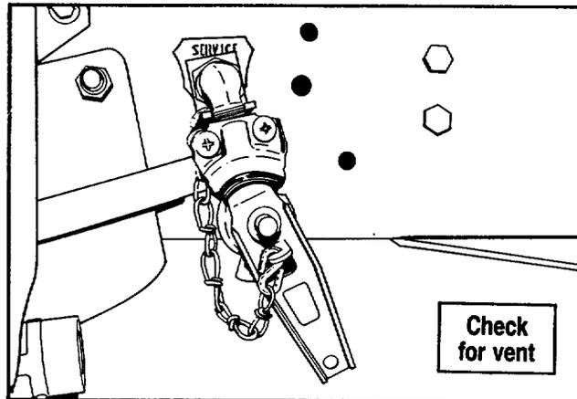
3. That's because the service dummy coupling needs a breather vent to release air pressure. If you have the right coupling and the brakes lock up, the vent hole may be plugged with dirt or paint.
