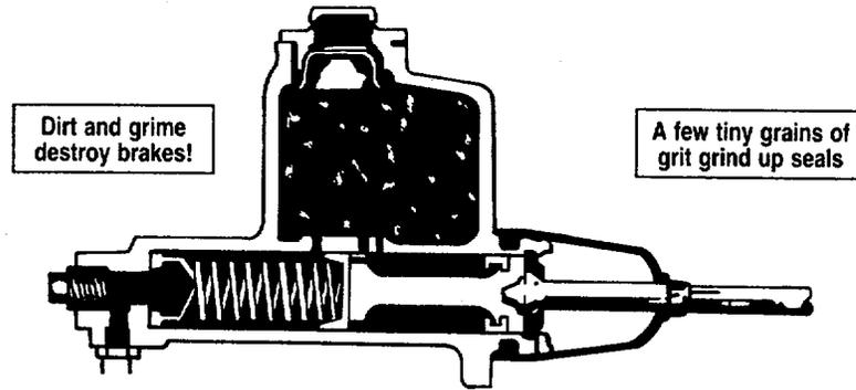
3. Grit and dirt usually sneak into the brake system when you check or add fluid. This is true for all vehicles, but the problem is worse on 2 1/2- and 5-ton trucks. Dirt has more chances to get into the brake system because the master cylinder is located underneath the trap door in the floorboard..
