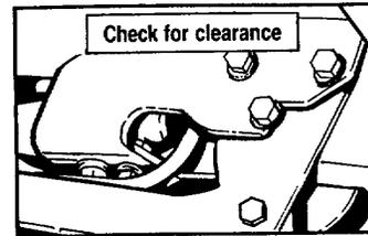
3. If there's not enough clearance, move the hose gently. Bend the brake line at the "T" and turn the hose clamp on top of the rear suspension arm. You must be careful not to move them more than they need.
