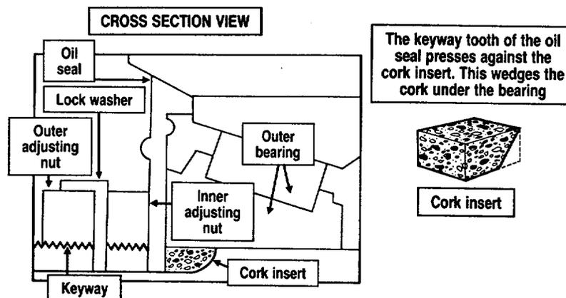
5. Oil in the axle housing travels out to the end of the axle housing spindle. The outer seal blocks this oil from getting into the hub, except where the spindle keyway provides a handy channel under the outer bearing.
