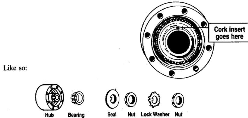
The cork insert is jammed under the bearing by the seal keyway tang when pressure is applied to the nut.
