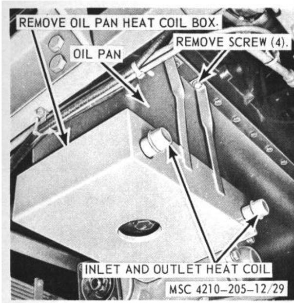
**Figure 29. Oil pan heater adapter, removal and installation.**
