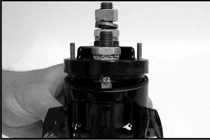
the link spool in the switch plunger and torque to 54-66 lbf-in. Grip the plunger either in soft jaws in a vise or using a pipe wrench and a strip of emery cloth to grip the plunger. Ensure that no nicks or burrs are raised during this operation. Figure 29
